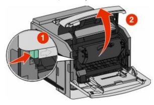
**3** Lift and pull the print cartridge out of the printer.
