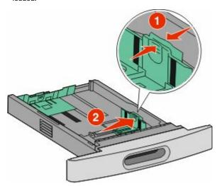
**3** Unlock the length guide, squeeze the length guide tab inward as shown, and slide the guide to the correct position for the paper size being loaded.
