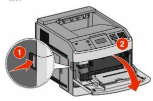
**2** Push the release latch, and then open the front cover.
